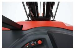
An angled front cover enhances visibility so that operators can see what they are moving, right down to the floor.
