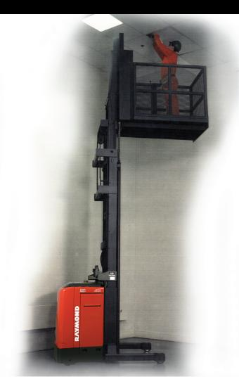
The *Raymond* Electric Maintenance Platform Vehicle, Model MPV, is built to the following specifications and conforms to ANSI A92.6 1990:
