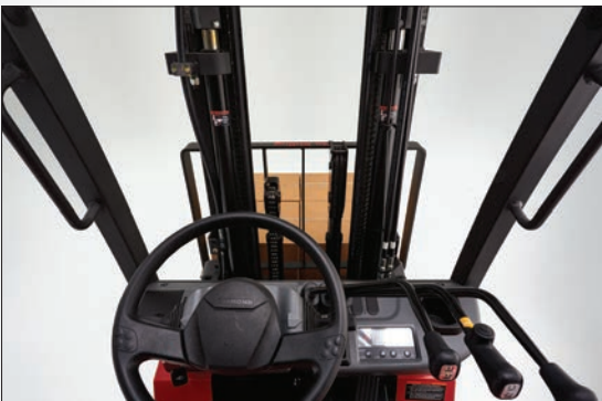
Open view mast provides operators with the best line of sight for the task at hand.
