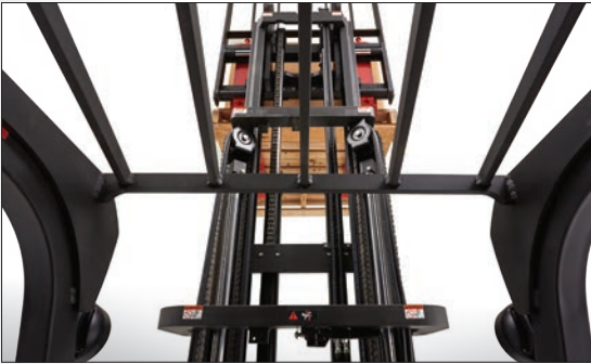
Overhead guard design provides operators greater visibility at elevated heights.
